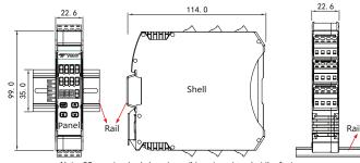
Note: 35mm standard clamping rail is not equipped at the factory, and the product must be fixed on the clamping rail for use.
